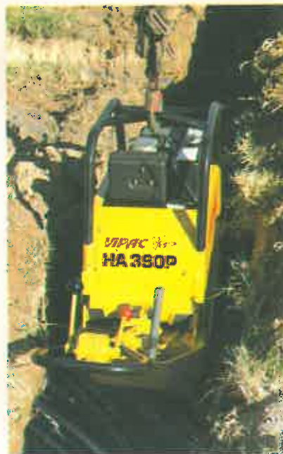
The new lifting frame enabling safe and easy access to trenches.
